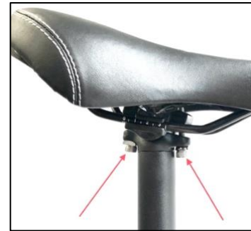
Fig. 7 c. Use silver bolts to adjust seat
