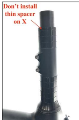
Fig. 13 f. Slide stem extender and spacers onto steering tube
