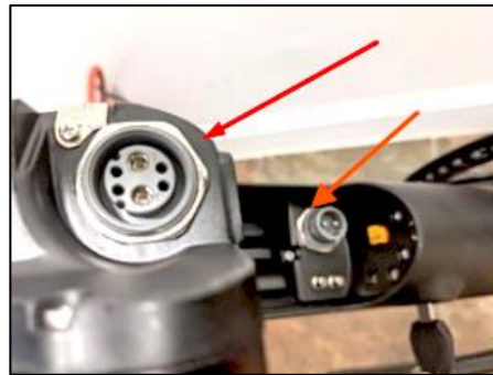
Fig. 10 b. Tighten silver lock rings
