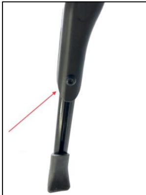
Fig. 8 b. Kickstand length adjustment bolt
