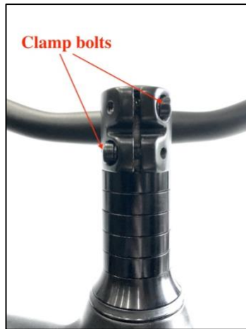
Fig. 13 d. Loosen rear stem clamp bolts
