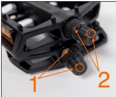
Fig. 6 a. Identify right (1) and left (2) pedals
