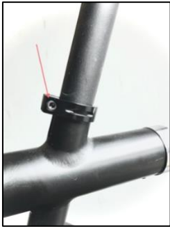
Fig. 7 a. TYPE 1: Loosen single bolt to install seatpost and adjust height
