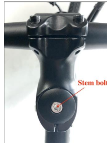
Fig. 13 e. Loosen stem bolt and remove with top cap
