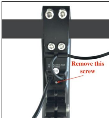
Fig. 13 i. Remove small screw to remove display from stem
