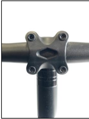
Fig. 2 c. Replace and tighten clamp bolts evenly
