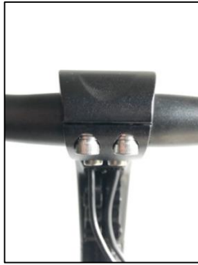
Fig. 2 f. Replace and tighten clamp bolts evenly
