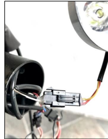
Fig. 5 c. Plug light into power cable connector
