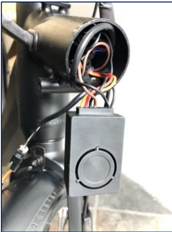
Fig. 5 a. If necessary, remove alarm box to access power cable
