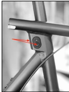
Fig. 7 b. TYPE 2: Loosen 2 bolts to install seatpost and adjust height
