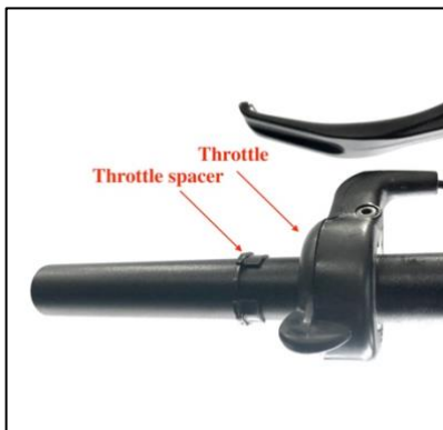
Fig. 12 f. Remove left grip and slide throttle spacer on after throttle
